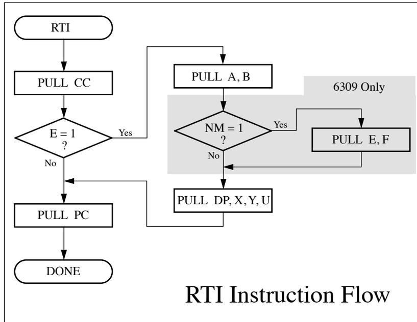
Interrupt service routines should strive to use the RTI instruction for returning control to the interrupted task. All the logic for proper restoration of the machine state, based on the CPU's current execution mode, is built-in.
