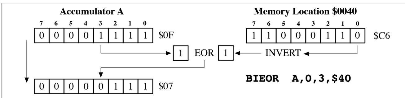
The figure above shows an example of the BIEOR instruction where bit 3 of Accumulator A is Exclusively ORed with the inverted value of bit 0 from the byte in memory at address \$0040 (DP = 0).
