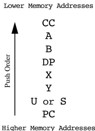
For each 8-bit register specified, the stack pointer is decremented by one and the register's value is stored in the memory location pointed to by the stack pointer. For each 16-bit register specified, the stack pointer is decremented by one, the register's low-order byte is stored, the stack pointer is again decremented by one and the register's high-order byte is then stored.
