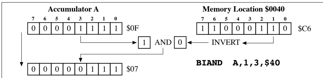
The figure above shows an example of the BIAND instruction where bit 3 of Accumulator A is ANDed with the inverted value of bit 1 from the byte in memory at address \$0040 (DP = 0).
