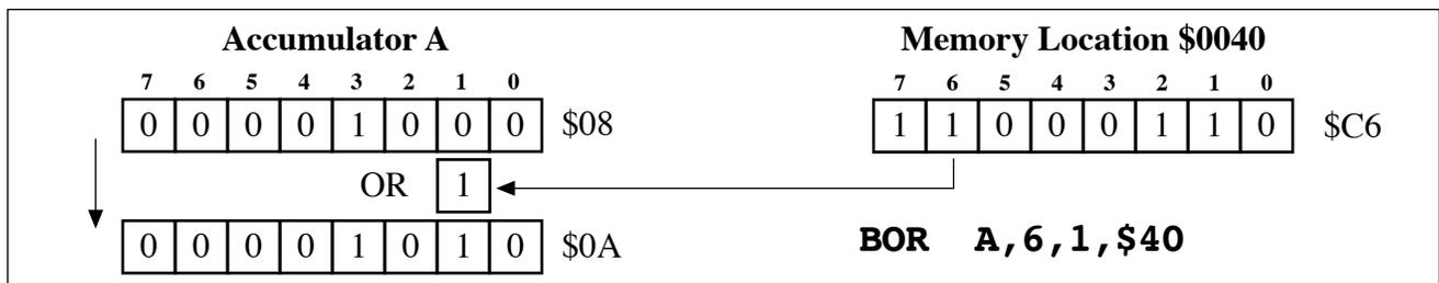
The figure above shows an example of the BOR instruction where bit 1 of Accumulator A is ORed with bit 6 of the byte in memory at address \$0040 (DP = 0).
