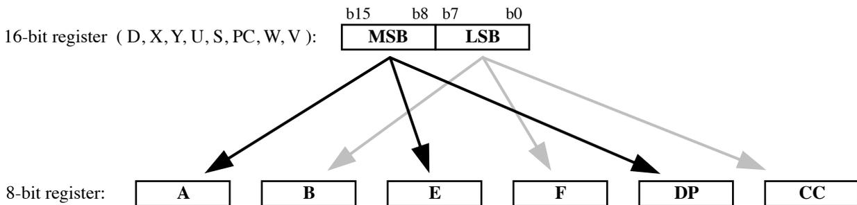
The TFR instruction requires a postbyte in which the source and destination registers are encoded into the upper and lower nibbles respectively.
