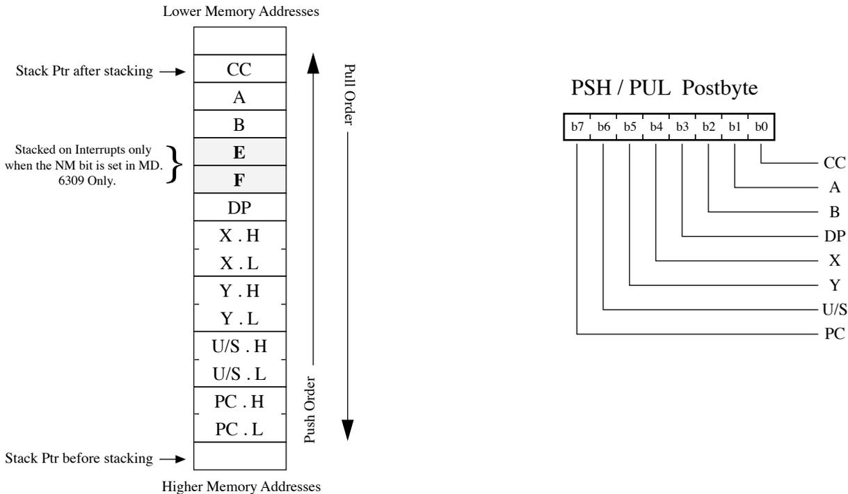
When the FM bit in the MD register is set, the Entire register set is stacked upon an FIRQ interrupt, otherwise only CC and PC are stacked.
