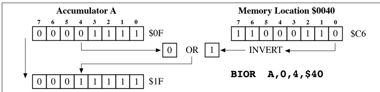
The figure above shows an example of the BIOR instruction where bit 4 of Accumulator A is logically ORed with the inverted value of bit 0 from the byte in memory at address \$0040 (DP = 0).
