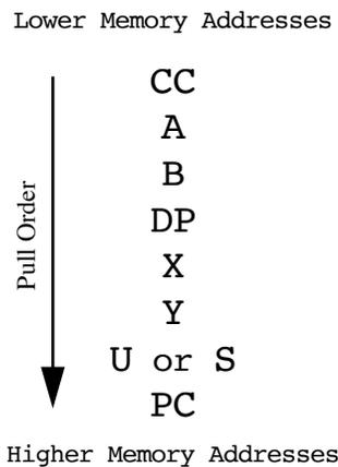
For each 8-bit register specified, a byte is read from the memory location pointed to by the stack pointer and then the stack pointer is incremented by one. For each 16-bit register specified, the register's high-order byte is read from the address pointed to by the stack pointer and then the stack pointer is incremented by one. Next, the register's low-order byte is read and the stack pointer is again incremented by one.
